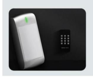
Equip with a remote control can set the Wiegand output from 26~44, 56, 58bits
