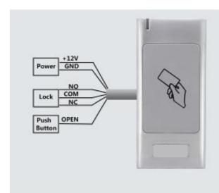
6 wires, easy installing
