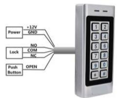
6 wires only, Easy to install and operate
