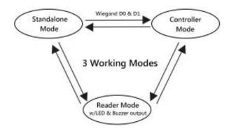
Three working modes-Wiegand 26~37 bits input & output
