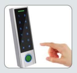
Backlit keypad,can set automatic OFF after 20 seconds Tri-color LED status display Wet finger also can touch keypad
