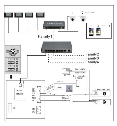
**Note:** Optional for POE function Outdoor station not need extra power supply when with built-in POE function.
