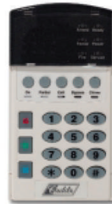
NV-2508S with door removed
